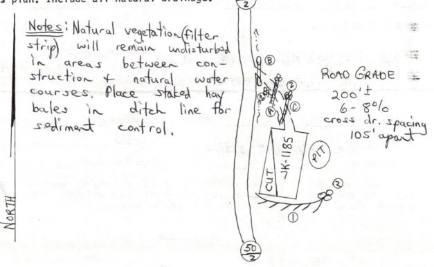
Drilling pit may vary in location other than that shown on this plan and/or other pits may be added due to soil type, newly discovered water systems, and the encounter of rock when building location.
