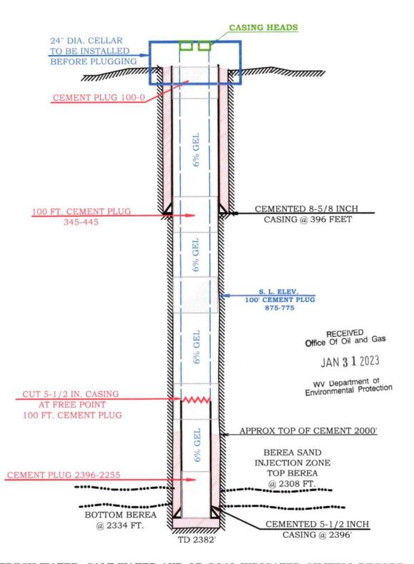
NO FRESH WATER, SALT WATER AND OR COAL INDICATED ON WELL RECORD. NOTE: TOTAL DEPTH ON FORMATION 2382, PIPE SCHEDULE INDICATES 2396 CASING WW-4A Revised 6-07 PRECEIVED
