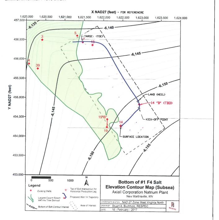
Figure 2. Contour Plot of the Subsea Elevations for the Bottom of the #1 F4 Salt.
