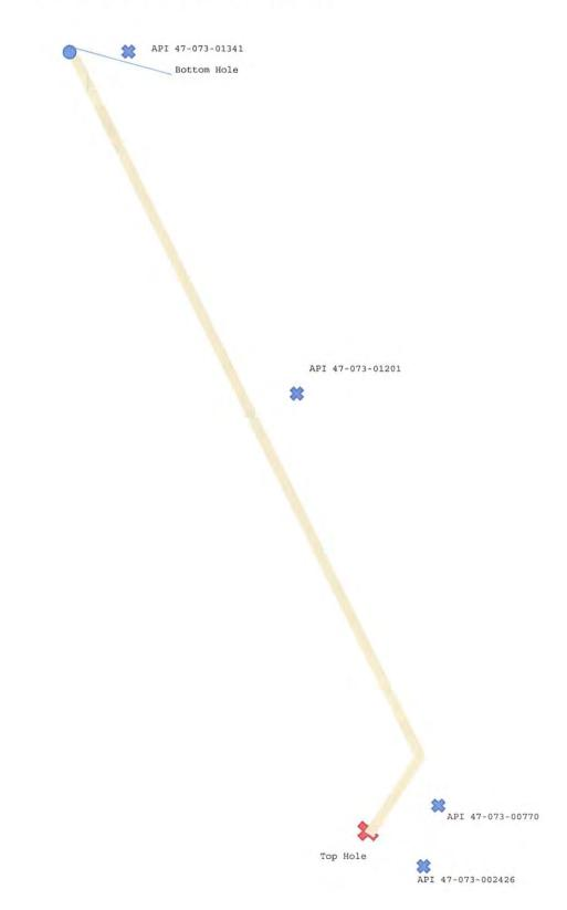
Well-Site Safety Plan Anti-Collision Schematic
