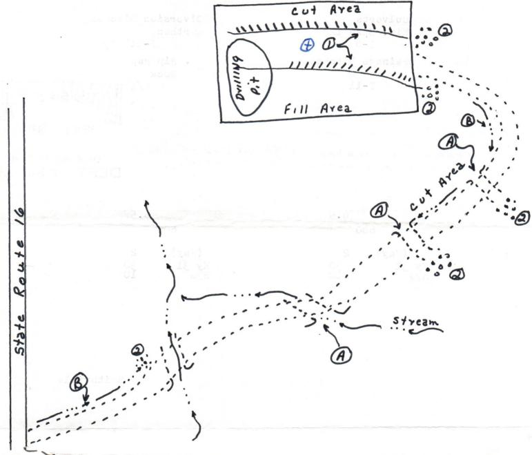
Comments: Slope on well road to be approx 15%. All disturbed areas to be seeded and mulched. Cuts of be on a 2:1 slope or less Diversion ditches and drainage ditches along road will be
