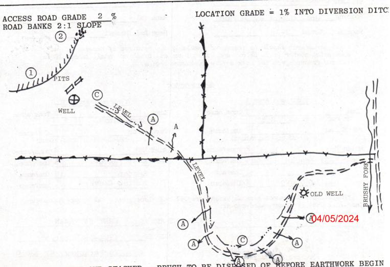
TREES TO BE CUT AND STACKED. BRUSH TO BE DISPOSED OF BEFORE EARTHWORK BEGIN REVEGETATION TO BE COMPLETED WITHIN SIX MONTHS OF WELL COMPLETION.
