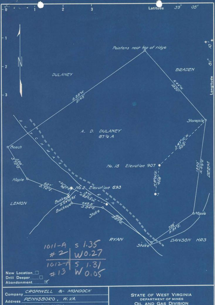
Farm A. D. DULANEY \_\_\_\_\_ Acres 87 2 Lease No.\_ Tract\_\_ Well (Farm) No. 2 & /3 \_Serial No. Elevation (Spirit Level) 693 & 907 Quadrangle HARRISVILLE County\_\_\_RITCHIE\_\_\_\_District\_\_MURPHY Engineer B. F. RINEHART Engineer's Registration No. 648 \_\_Drawing No. <u>797- MR</u> File No.\_\_ Date Nov. 9, 1950 Scale\_1 in.= 400 ft.
