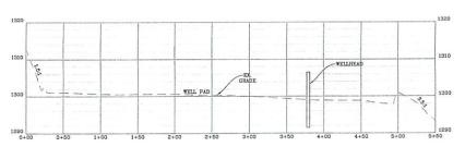
WELL PAD AS-BUILT CROSS-SECTION "A-A"
