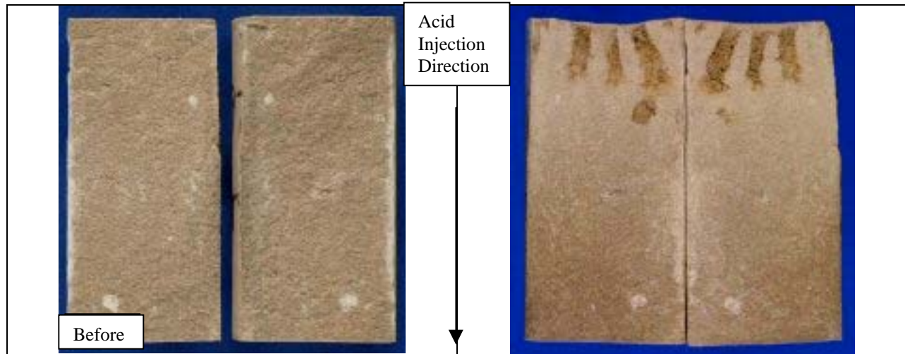
FIGURE 3 FLUID RESPONSE TESTING HARDY #14 WELL PLUG TT, 1397.4 FEET
