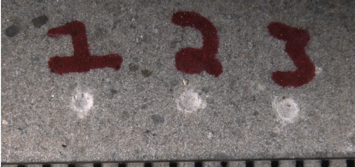
15% HCl Exposed Surface (Sample KK)
