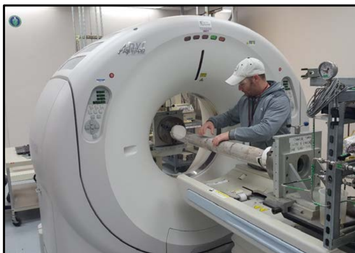
Figure 48: Toshiba® Aquilion™ Multislice Helical Computed Tomography Scanner at the NETL used for core analysis.
