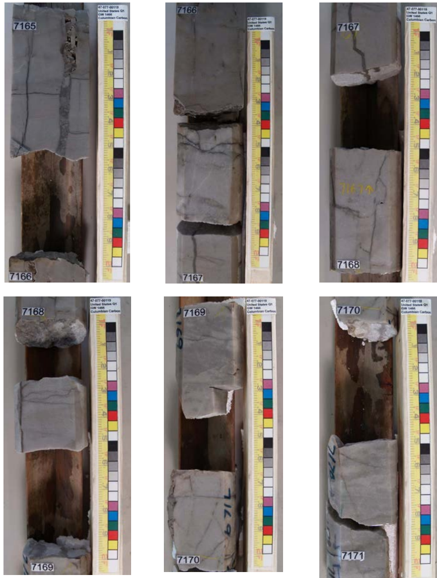
Figure 2: Pres-119 core photographs, from 7,165 to 7,171 ft.
