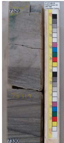
Figure 29: Pres-119 core photographs, from 7,326 to 7,332 ft.
