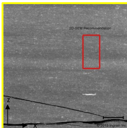
XCT Image Resolution - 4 \mu\text{m} per pixel Location #3 is recommended for 2D-SEM See attached image file : ARMSTRONG-1-9-7740P45_4X_TILE
