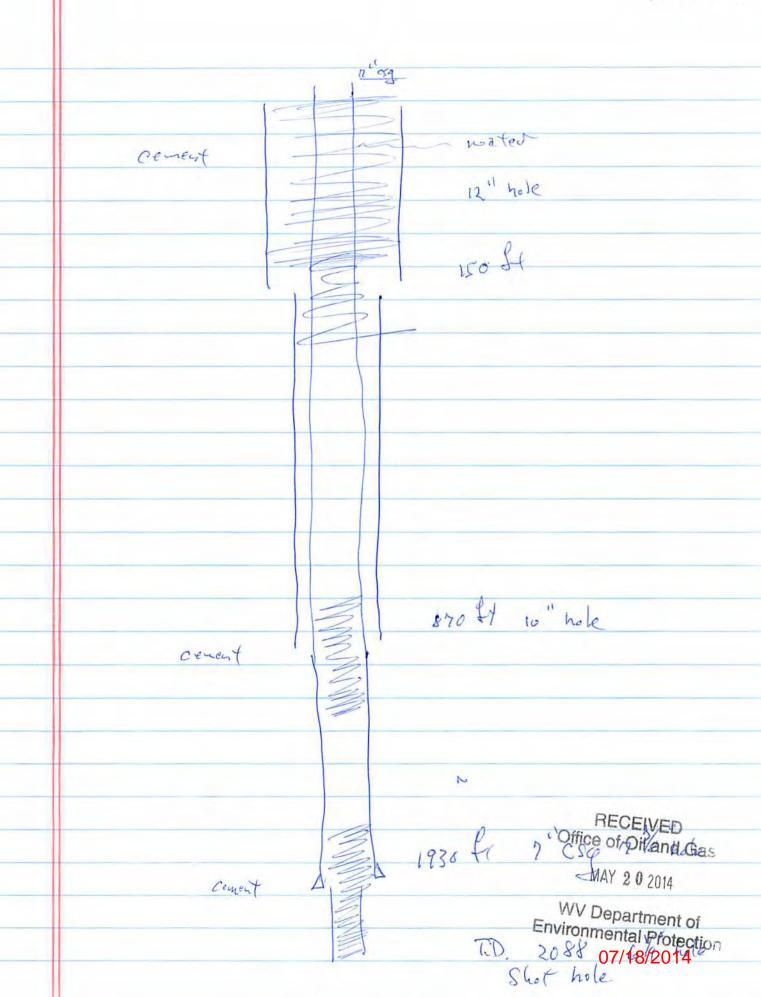
MIRU - Pull tubing & Rody -2 3 -trip work string in hole & spot cement from 4 J.D. to 1870 ft.
