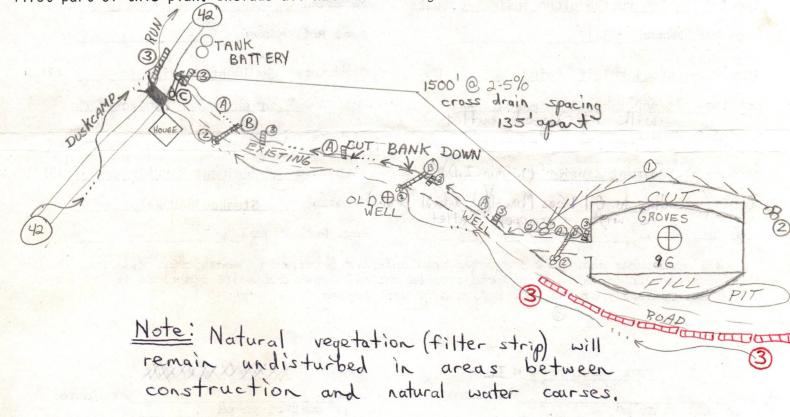
Access road subject to change between company and land owner, or aquirement of right-of-way. If change is made, a revised reclamation plan will be submitted. All cuts 2:1 slope. All topsoil to be stockpiled and used in reclamation. All grades for roads and locations as well as sediment structures shown on drawing.
