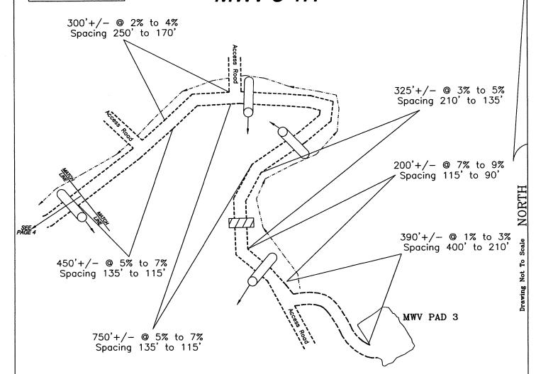
Road Is Existing. Upgrade Drainage Devices Where Needed.
