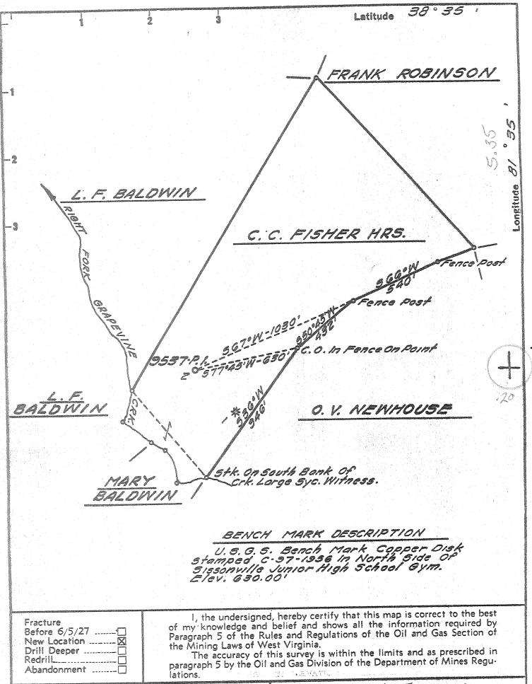
Company UNITED FUEL GAS CO. CHARLESTON, W. VA. Farm C. C. FISHER HRS. ET. AL. Acres 299 Lease No. 47510 ET.AL. Well (Farm) No. 2 Serial No. 9537 P.V. 830.22' Elevation (Spirit Level) \_ KENNA Quadrangle \_ County KANAWHA District 2330 Engineer's Registration No. File No. 64-69 Drawing No. Date APRIL 29,69 Scale 1"=400'
