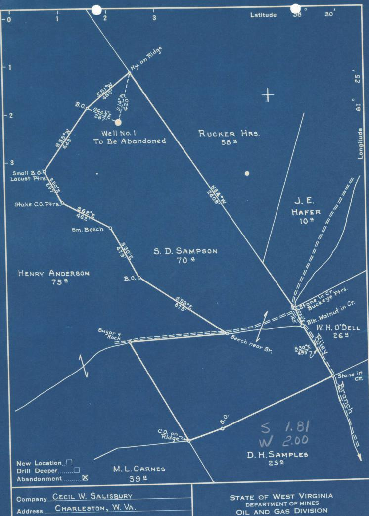
Farm S. D. SAMPSON Tract\_\_\_\_\_\_ Acres\_\_\_\_70\_\_\_Lease No. <u>13017</u> Well (Farm) No. \_\_\_\_ | Serial No. F5393 Elevation (Spirit Level) \_\_\_\_988.6 Quadrangle CLENDENIN County KANAWHA District ELK Engineer PAUL E. JOACHIM Engineer's Registration No. 669 File No. 70-67 Drawing No. . Scale 1" = 400'
