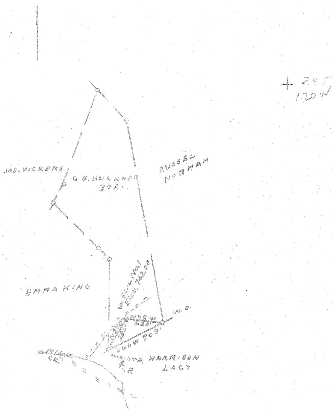
Minimum Error of Closure  $1' / \sqrt{200}$ Source of Elevation Fogles Road West 708.00
