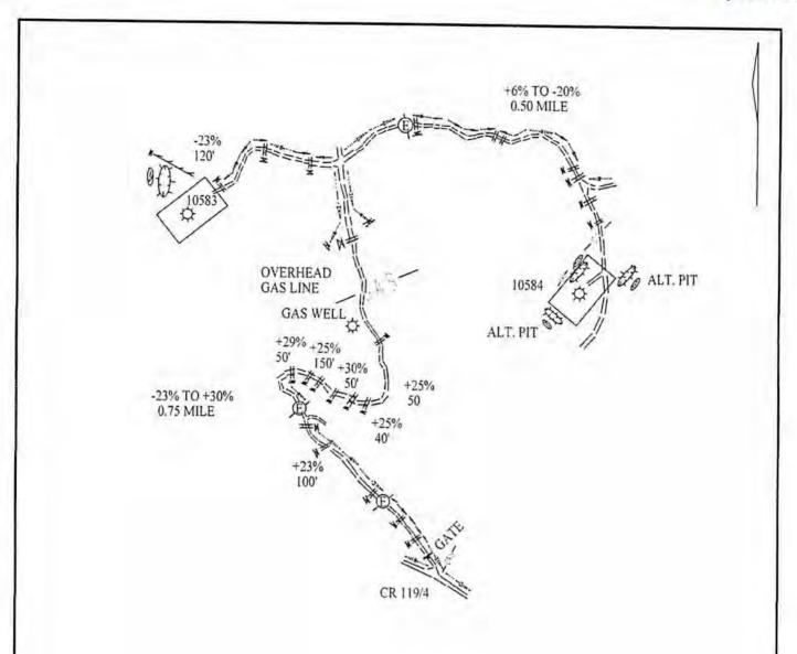
THIS PLAN IS FOR THE PLUGGING OF AN EXISTING WELL. ENTIRE LENGTH OF ACCESS IS EXISTING WELL ROAD. ROCK WILL BE USED WHERE NECESSARY.
