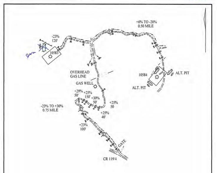
THIS PLAN IS FOR THE PLUGGING OF AN EXISTING WELL. ENTIRE LENGTH OF ACCESS IS EXISTING WELL ROAD. ROCK WILL BE USED WHERE NECESSARY. DRAWINGS TO ACCOMPANY FORM WW-9
