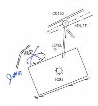
THIS PLAN IS FOR THE PLUGGING OF AN EXISTING WELL. ACCESS ROAD LEAVES CR 11/5 AT A GRAVEL DRIVEWAY AND WILL PROCEED ACROSS A GRASSY AREA TO THE WELL. ROCK WILL BE USED WHERE NECESSARY.
