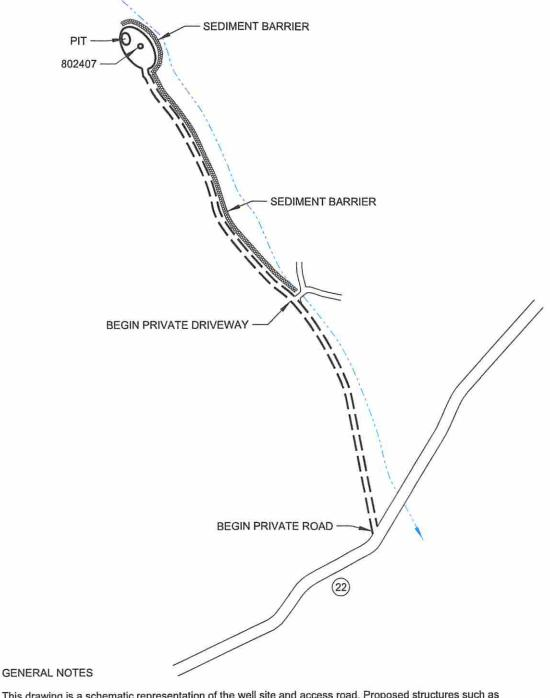
This drawing is a schematic representation of the well site and access road. Proposed structures such as well site, drilling pit, roadways, culverts, sediment barriers, etc. are show in approximate pre-planning configurations.
