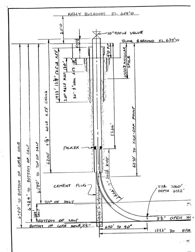
CONDUCTER PIPE - 30" A-53, 118.7 LB/PT, 68' SET, NOT CEMENTED, WELDED FRESH WATER PIPE - 20" H-40, 94 LB/FT, 130' SET, CEMENTED TO SURFACE, 8 RND THAD. & COUPLED, WELDED
