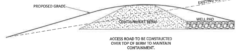
STANDARD CONSTRUCTION DETAIL MOUNTABLE BERM NTS
