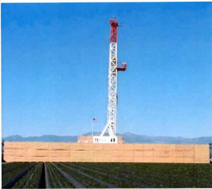
Figure 1. A sound blanket surrounding the drill rig would not work very well for obvious reasons.
