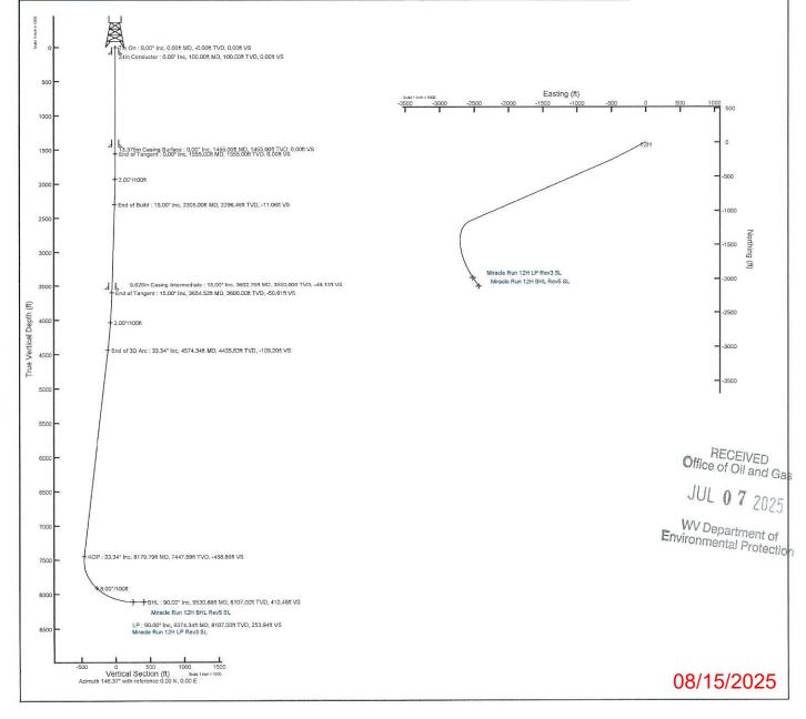
Operator's Well No. Miracle Run 12H
