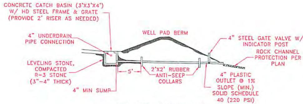
WELL PAD TYPICAL SUMP CROSS SECTION
