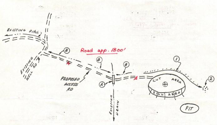
Cross ditches and/or culverts at appropriate locations, or about 250' spart.
