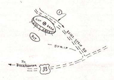
Comments: Slope of access road 1-2% -- cuts on a 2:1 slope or less -- because of flat terrain on strip only drainage ditch is needed -- access road subject to change between company and landowner.
