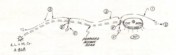
Comments: Slope of access road 18% -- cuts to be on a 2:1 slope or less-- ditches to be maintained after construction is completed -- Reclamation to be performed by Hall Reclamation, Inc. -- access road subject to change between landowner or company
