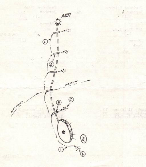
Comments: Slope of access road 5% -- Cuts to be on a 2:1 slope or less -- Access road subject to change by company or landowner -- All ditches and culverts will be maintained after construction is completed -- Reclamation to be performed by Halls Reclamation, Inc.
