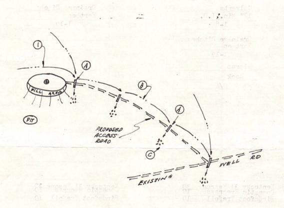
Comments: Slope of access road . 18% -- Cuts to be on a 2:1 slope or less -- Access road subject to change by company or landowner -- All ditches and culverts will be maintained after construction is completed -- Reclamation to be performed by Halls Reclamation, Inc.
