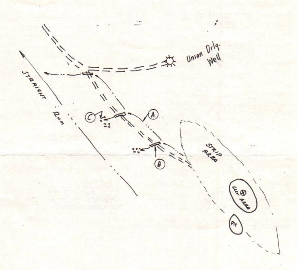
Comments: Slope of access road 11% -- Cuts to be on a 2:1 slope or less -- Access road subject to change by company or landowner -- All ditches and culverts will be maintained after construction is completed -- Reclamation to be performed by Halls Reclamation, Inc. -- location falls on strip no major drainage needed
