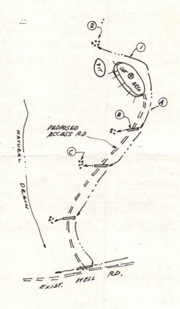
Comments: Slope of access road 25% -- Cuts to be on a 2:1 slope or less -- Access road subject to change by company or landowner -- All ditches and culverts will be maintained after construction is completed -- Reclamation to be performed by Halls Reclamation, Inc.
