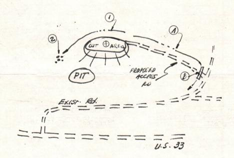
Comments: Slope of access road 10% -- Cuts to be on a 2:1 slope or less -Access road subject to change by company or landowner -- All ditches and culverts will be maintained after construction is completed -- Reclamation to be performed by Halls Reclamation, Inc.
