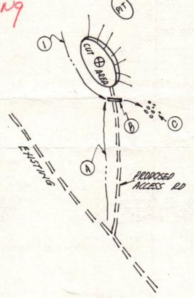
Comments: Slope of access road 18% -- Cuts to be on a 2:1 slope or less -- Access road subject to change by company or landowner -- All ditches and culverts will be maintained after construction is completed -- Reclamation to be performed by Halls Reclamation, Inc.
