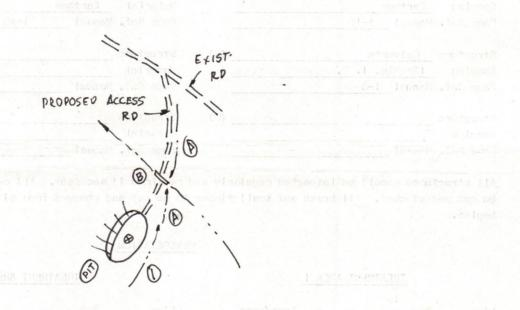
COMMENTS: Slope of access road 5% -- Cuts to be on a 2:1 slope or less -- Access road subject to change by company or landowner -- All ditches and culverts will be maintained after construction is completed -- Reclamation to be performed by Halls Reclamation, Inc.
