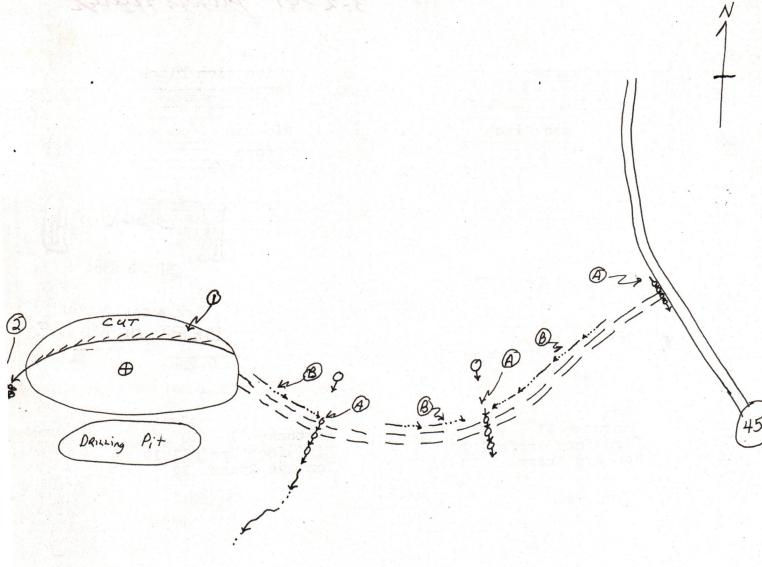
Comments: Cuts on a 2:1 slope. Road location subject to change. Mair culverts and ditches after completion. Timber 8" and up to be cut old pasture and woodland. P.O. Box 48 Buckhannon, WV 26201 472-940 and stacked Phone Number Signature: Address
