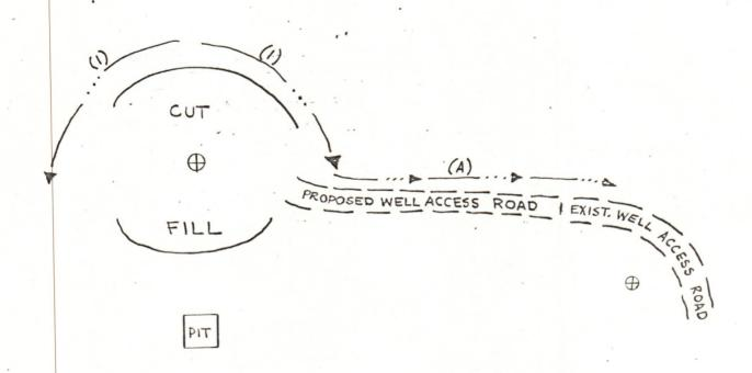
COMMENTS: Roadways will be cut with a maximum slope of 15% side cuts will be at a 2:1 ratio.
