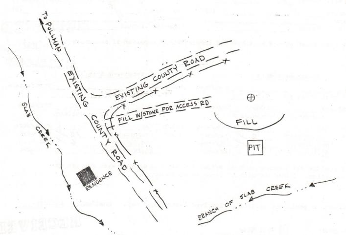
COMMENTS: Acces road and portion of well site will be stabilized with stone fill. Well road will be maintained after well is completed.
