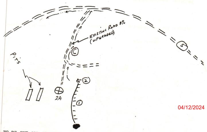
ES TO BE CUT AND STACKED. BRUSH TO BE DISPOSED OF BEFORE EARTHWORK BEGINS. EGETATION TO BE COMPLETED WITHIN SIX MONTHS OF WELL COMPLETION.
