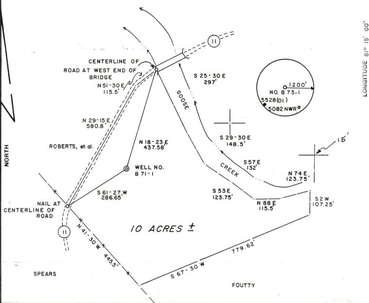
FILE NO .\_ DRAWING NO .\_ 1" = 200 MINIMUM DEGREE OF ACCURACY\_ PROVEN SOURCE OF ELEVATION JUNCT. OF ROADS ELEV. 779'
