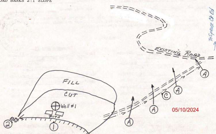
TREES TO BE CUT AND STACKED. BRUSH TO BE DISPOSED OF BEFORE EARTHWORK BEGINS. REVEGETATION TO BE COMPLETED WITHIN SIX MONTHS OF WELL COMPLETION.
