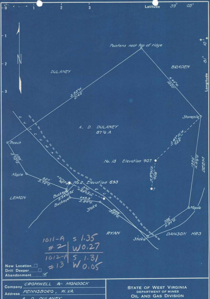
Farm A. D. DULANEY Well (Farm) No. 2 & 15 \_Serial No.\_ Elevation (Spirit Level) 693 & 907 Quadrangle HARRISVILLE County RITCHIE District MURPHY Engineer B. F. RINEHART Engineer's Registration No. 648 \_Drawing No. 797- MR File No.\_ Scale 1 in. = 400 ft. Date Nov. 9, 1950
