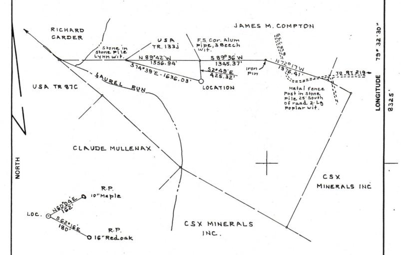
FILE NO. BK 95 P 92 DRAWING NO. SCALE \_ 1"= 1000' MINIMUM DEGREE OF ACCURACY\_1: 200 PROVEN SOURCE OF ELEVATIONUSGS BM at Jct RTS 219 & 9 E1 3289
