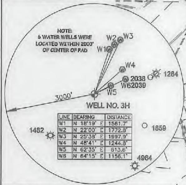
NOTE: 6 WATER WELLS WERE LOCATED WITHIN 2000' OF CENTER OF PAD
