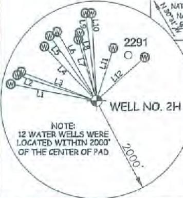
NOTE: 12 WATER WELLS WERE LOCATED WITHIN 2000' OF THE CENTER OF PAD
