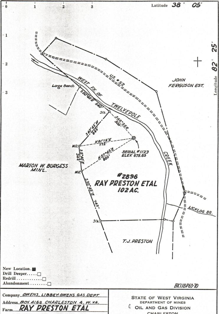
Acres 102 Lease No. 2896 Serial No. //23 Well (Farm) No. / 675.85 Elevation (Spirit Level)\_\_ WAYNE Quadrangle\_\_\_ WAYNE District LINCOLN T. S. FLOURNOY Engineer\_\_ Engineer's Registration No.\_ File No. \_\_Drawing No. Date AUG. 25, 1960 Scale /" = 400 FT.
