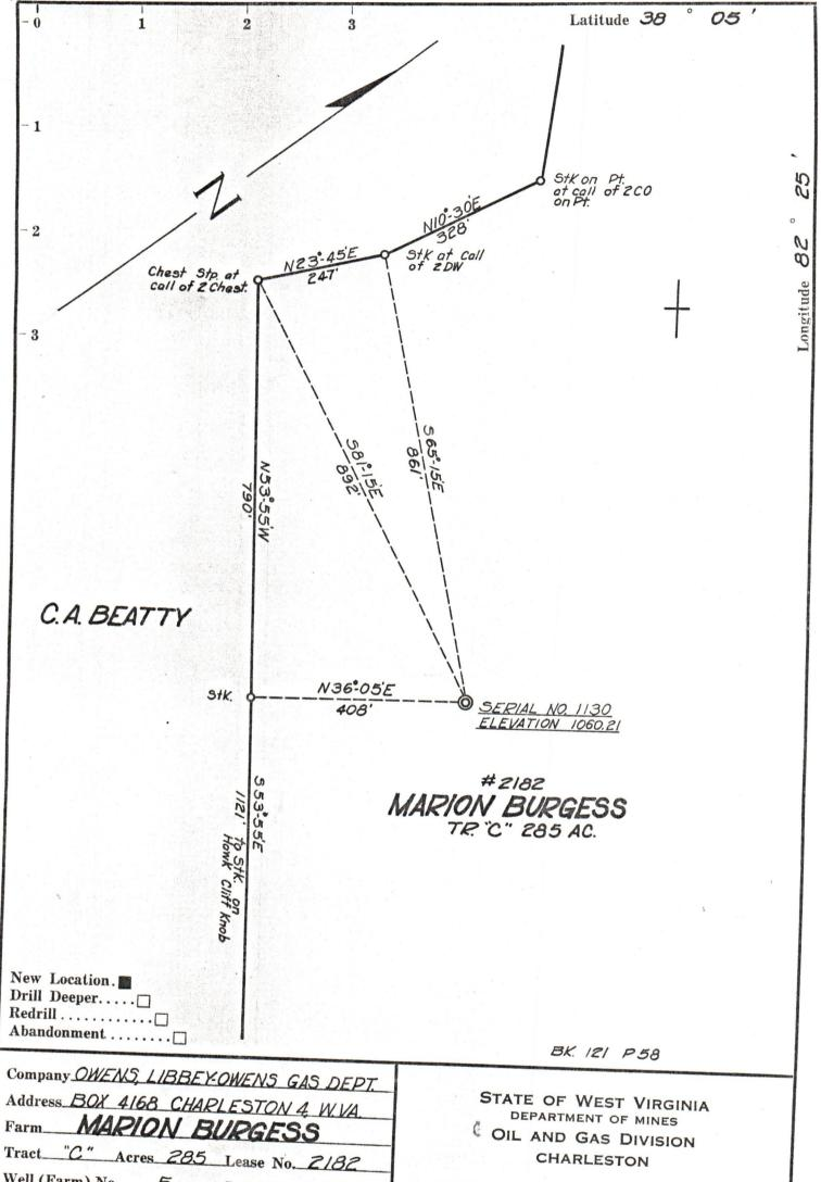
Well (Farm) No. 5 Serial No. 1130 Elevation (Spirit Level) 1060.21 Quadrangle\_WAYNE County\_\_\_WAYNE District LINCOLN Engineer T. S. FLOURNOY Engineer's Registration No.\_\_ File No. Drawing No. Date MAY 25, 1961 Scale /=200 FT. ALLEN BLUEPRINT & SUPPLY CO
